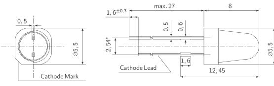
all dimensions in mm. Tolerance  $\pm 0,\,1$  except given ones \* at the bottom of the LED
