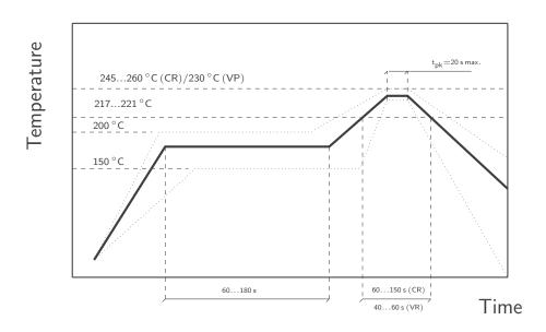
Recommended reflow soldering conditions following IPS/JEDEC J-STD-020.
