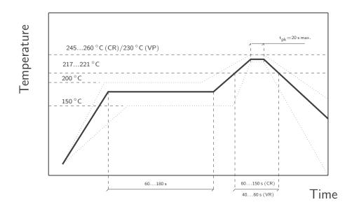
Recommended reflow soldering conditions following IPS/JEDEC J-STD-020.
