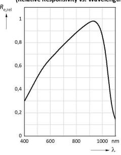
Blue enhanced PIN photodiode chip 120 mil
