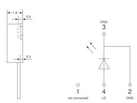
all dimensions in mm. Tolerance  $\,\pm$  0, 1 except given ones \* at the bottom of the LED
