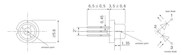
all dimensions in mm. Tolerance  $\pm {\rm 0}\,,$  2 except given ones \* at the bottom of the LED
