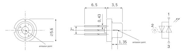
all dimensions in mm. Tolerance  $\pm 0,\,1$  except given ones \* at the bottom of the LED
