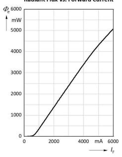
Radiant Flux vs. Forward Current
