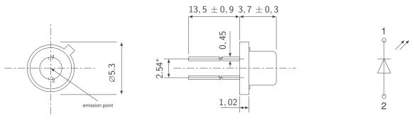
all dimensions in mm. Tolerance  $\pm {\rm 0}, {\rm 2}$  except given ones \* at the bottom of the LED
